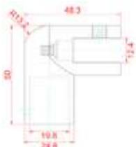
**GL-CN002****CONECTOR PARED TUBO AJUSTABLE**
