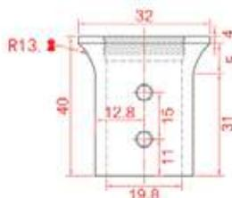
**GL-CN020****CONECTOR TUBO VIDRIO AJUSTABLE**
